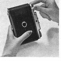
Close the camera back and advance the film until number "1" appears in the red aperture on the camera back.
